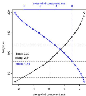
Figure 10 Along-wind and cross wind shear for a site in Great Plains. The “mean” horizontal wind vector is defined as the vector at 80 m.
