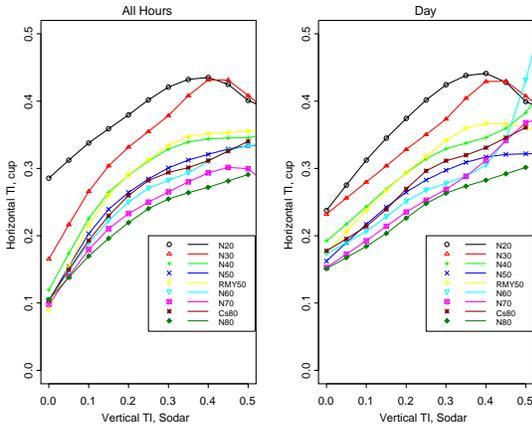
Figure 6 Horizontal TI from cup anemometers as a function of vertical TI from sodar for various heights from 20 m to 80 m.
