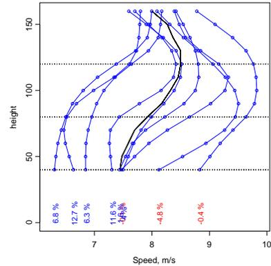
Figure 8 Sequence of wind profiles measured during a 1.5 hour period of downslope flow. Numbers on the bottom are percent deviation of the integrated rotor plane power from the power determined by the hub height wind speed. Red numbers depict a deficit of power, blue a surplus.
