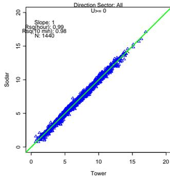
Figure 3 Scatter plot of hourly-averaged sodar 50 m wind speeds against tower 50 m wind speeds.
