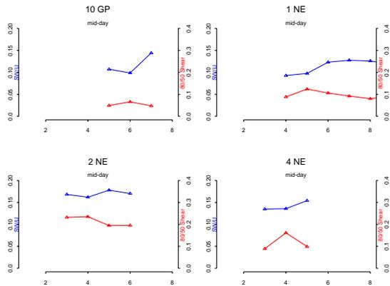
Figure 7 Vertical TI (blue lines) and 80/50 m shear parameter (red) for 4 sites during the spring transition. Numbers on the horizontal axis are month of the year.
