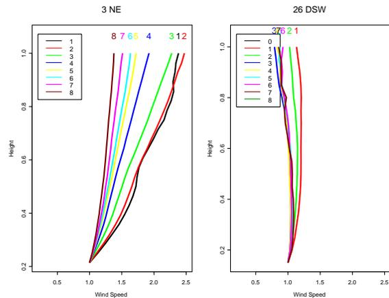
Figure 5 Normalized mean wind profiles by vertical TI category ( $=TI/0.05$ ) for two sites (left) in the desert southwest and (right) in the northeast.
