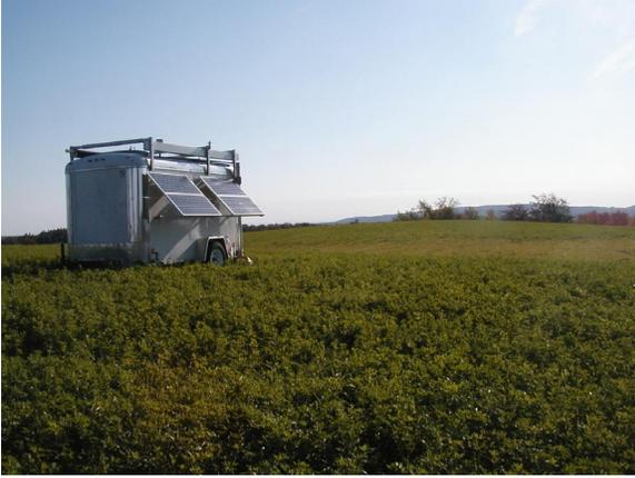
Figure 2 ART model VT-1 sodar in a trailer-mounted configuration.
